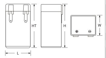
**L:** 1.69 (43) **W**: 1.46 (37) **H**: 2.99 (76) **HT**: 2.99 (76) Tolerances are +/- 0.04 in. (+/- 1mm) and +/- 0.08 in. (+/- 2mm) for height dimensions. All data subject to change without notice.
